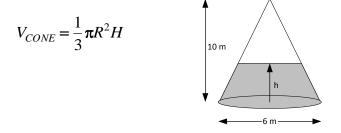
where R is the radius of the cone's base and H is the height of the cone-shaped tank. What is the volume of water in the tank when the height of the water is h?
